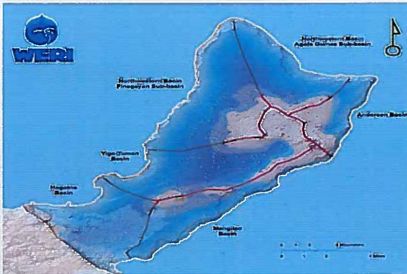
Fig.3. Revised contour map of the volcanic basement underlying the limestone plateau in northern Guam. Northern Watershed Sub-basins.
